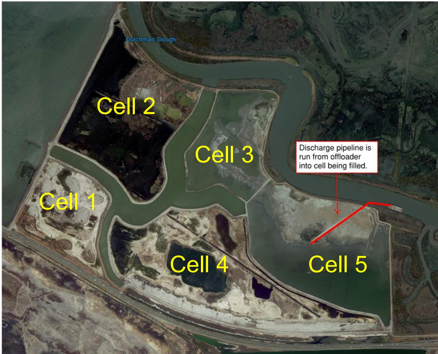
The dredge sediment is pumped hydraulically from the dump scow or hopper barge and placed into the selected cell. Material is pumped until design elevation is achieved.
