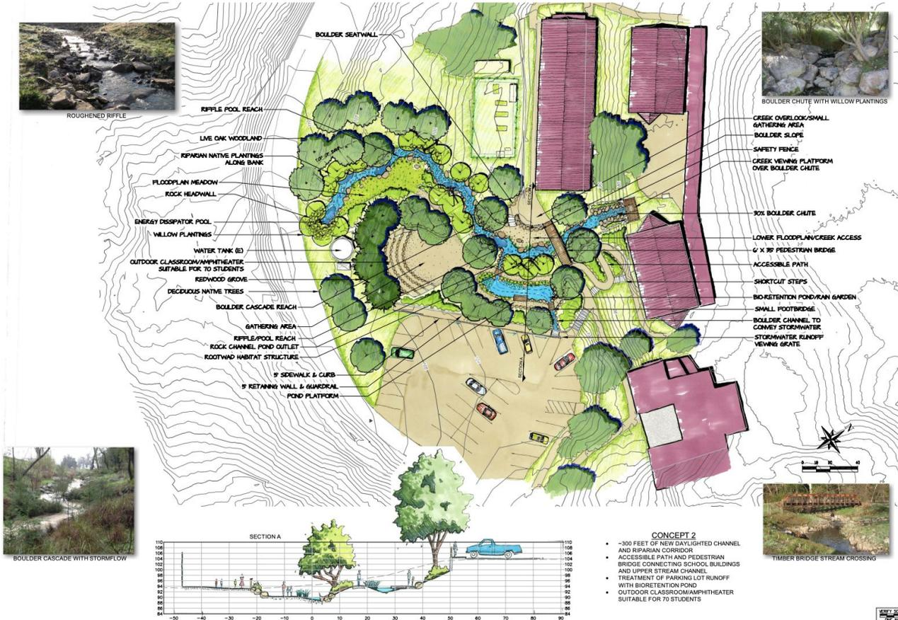
Willow Creek flows from its source, above Hwy 101, to the edge of Richardson Bay, running primarily underground in concrete culverts. **The Willow Creek Restoration Plan** is part of a phased process of “infrastructure renewal”, consistent with a shared community vision.
