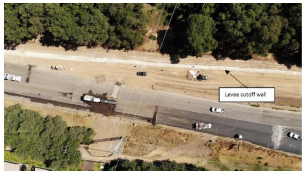
FO Monitoring of cement bentonite cut-off wall, currently upgraded.
